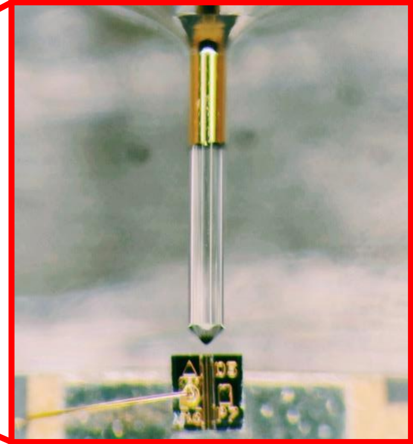
Microscope View of a Tapered Lensed Fibre Attached Using the Laser Welder
