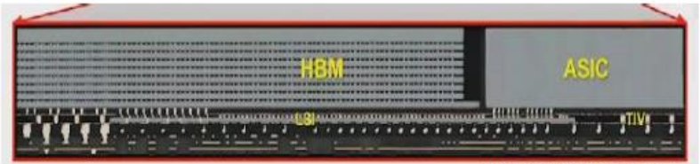
Figure 1: Schematic and cross-section of IBM's DBHi Si Bridge technology. (Courtesy of IBM) Source: IBM
