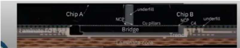
Figure 1: Schematic and cross-section of IBM's DBHi Si Bridge technology. (Courtesy of IBM) Source: IBM
